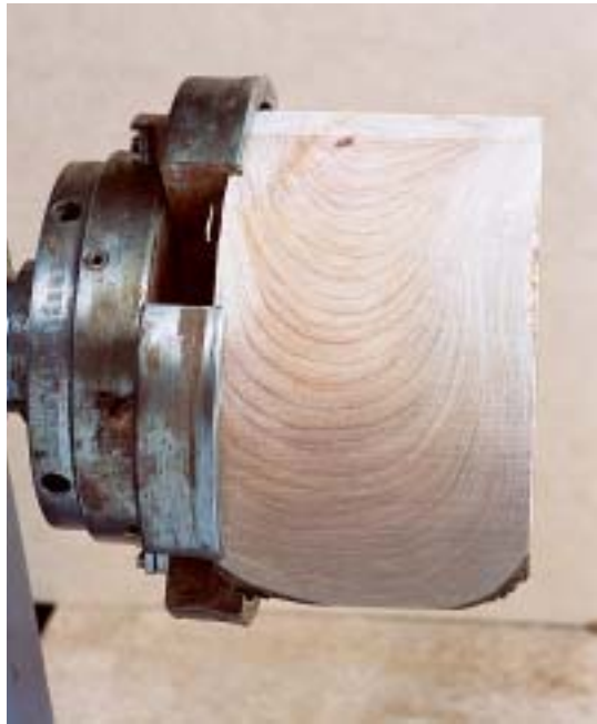
Small blanks can be conveniently gripped in a chuck to shape most of the bowl's profile. You can complete the rim when you remount the blank for hollowing.
