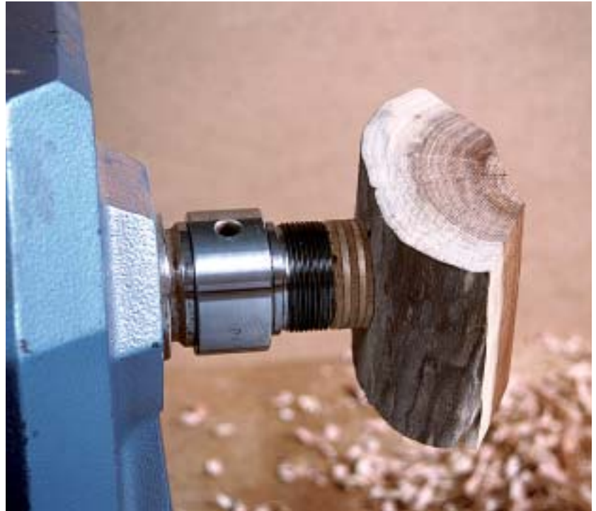
A small blank can be held on a very short screw, here about \frac{3}{8} in. (9mm) long.
