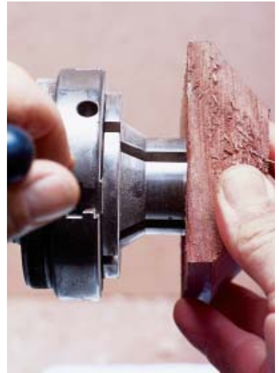
Expanding long-nose jaws within a drilled hole is a fast and simple way to grip a small blank.
