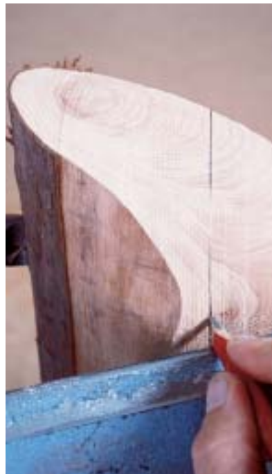
On blanks with a symmetrical round face, align the two-spur drive along the main axis of the curve on top of the blank. Mount the blank with the top at 90 degrees to the lathe axis and the sides evenly balanced. A pencil line drawn on the roughed bowl profile indicates how much the blank needs to be repositioned to bring the lower portions of the rim into the same plane (left, center). Make this adjustment easier by using the lathe to support your arm as you pivot the blank on the two-spur drive (above).
