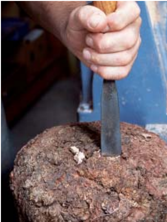
To mount a blank with an uneven surface between centers, chisel a V-groove to receive a two-spur drive (left). As you bring the tail center up, steady the blank by resting your arm on the tool rest (above).
