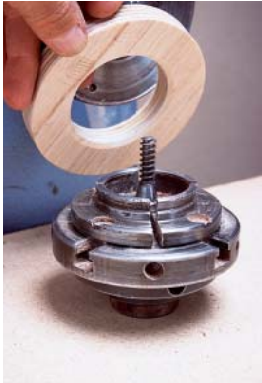
A turned washer broadens the face of a set of standard chuck jaws to provide a better grip for blanks above 6 in. (150mm) in diameter.
