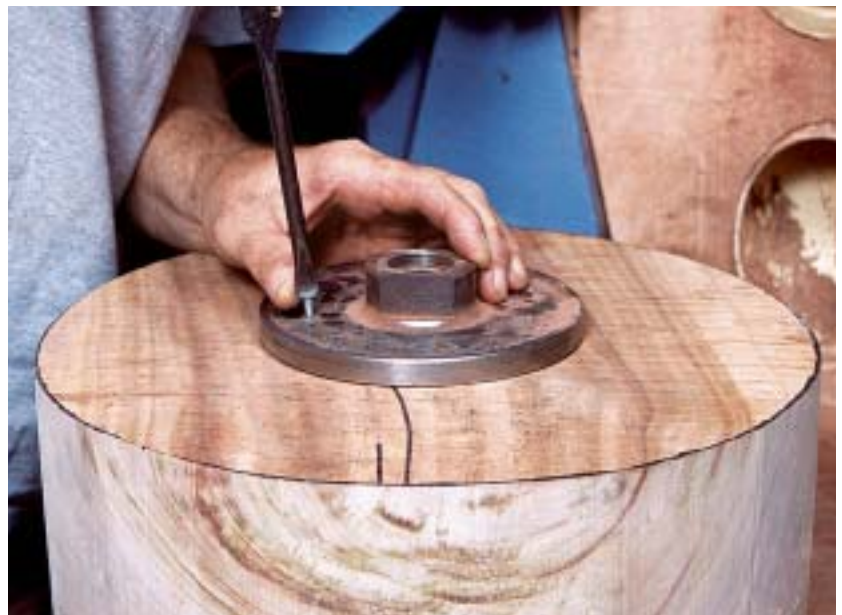
A faceplate is the most secure way to hold a blank on the lathe.
