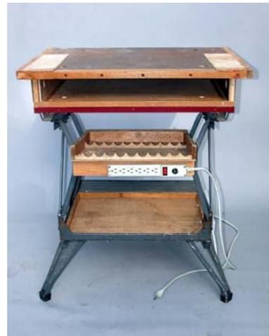
The Photo on the right shows the base assembly with the case for the drawer unit bolted to the top. The stand, with the step towards the front, is now ready to accept the tool drawer as shown in the next photo (open position).
