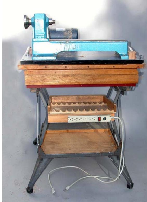
The front display tray is wedged below the lathe platform. All accessories such as the Tool Rest, Tailstock, Belt Guard, Lamp and the 18” high wrap around safety shield have to be added. This assembly is shown in the next picture
