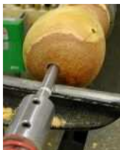
Straight tool first, it fits just in the hole.
