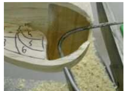
...to control the wall thickness.
