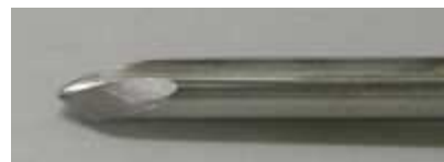
This grind works well for drilling the central hole.
