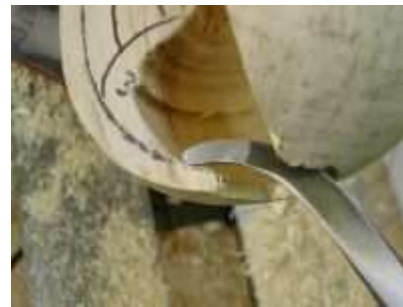
Final cut under the rim with the more curved tool.
