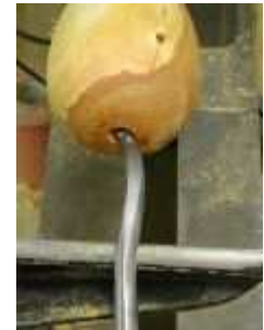
The toolrest is placed before the tool curve.
