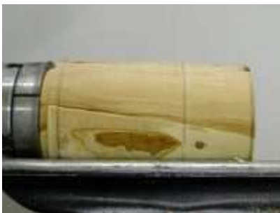
dimensions are marked on the wood held in the chuck.
