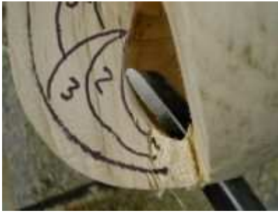
The tool is rolled on its side to take a light cut.
