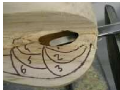
Widening the hole with the straight tool in zone 1.
