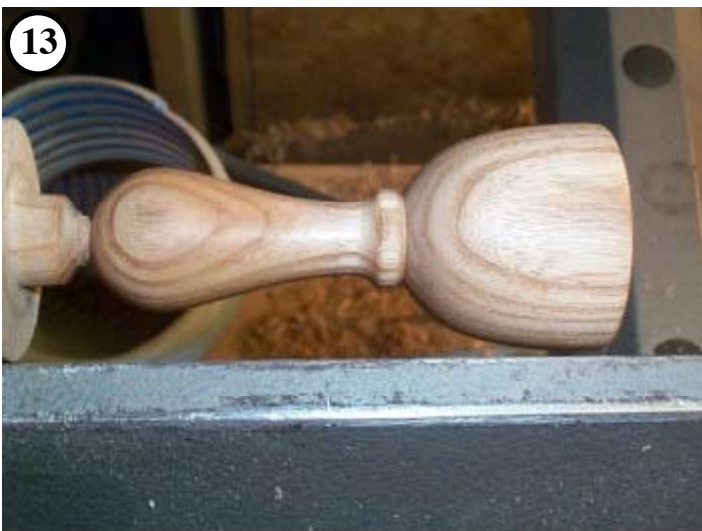
13 The piece is sanded and finished, ready for parting off.
