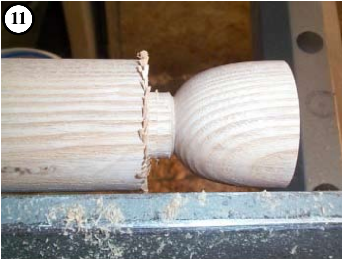
11 The outside of the cup has been shaped and is ready for sanding.
