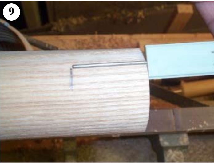
9 Here I am transferring the depth of the cup to the outside of the blank.
