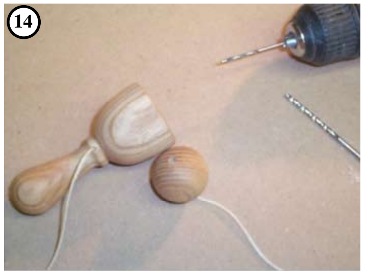
14 The toy is ready for play. I drill a 1/8" hole about half way through each part, then finish the hole with a 3/64" bit. This leaves a shoulder inside the hole so that a knotted string will not pull through.
